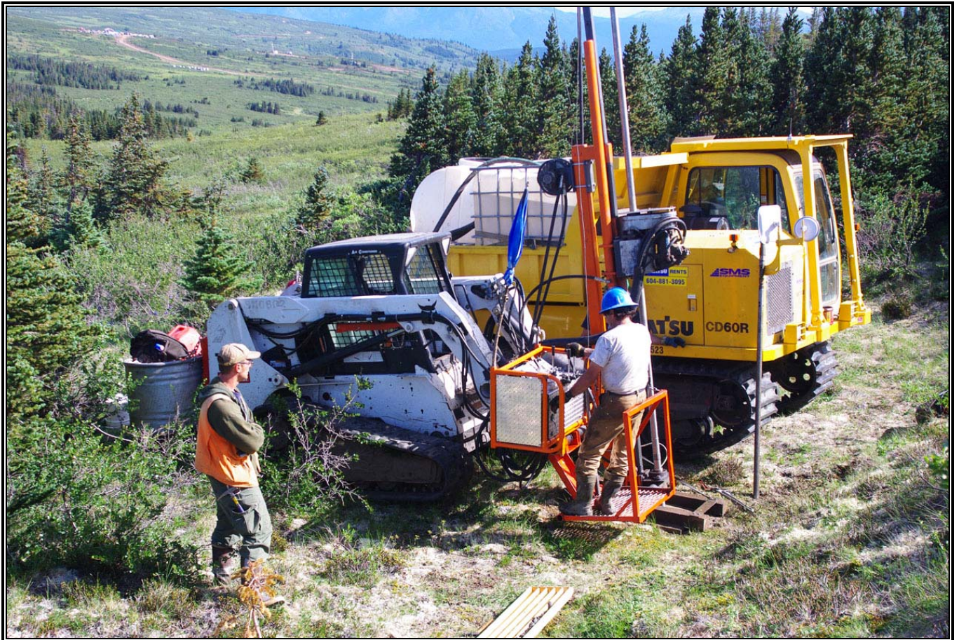
Figure 11.2 Bobcat Mounted Hydra Core Drill
