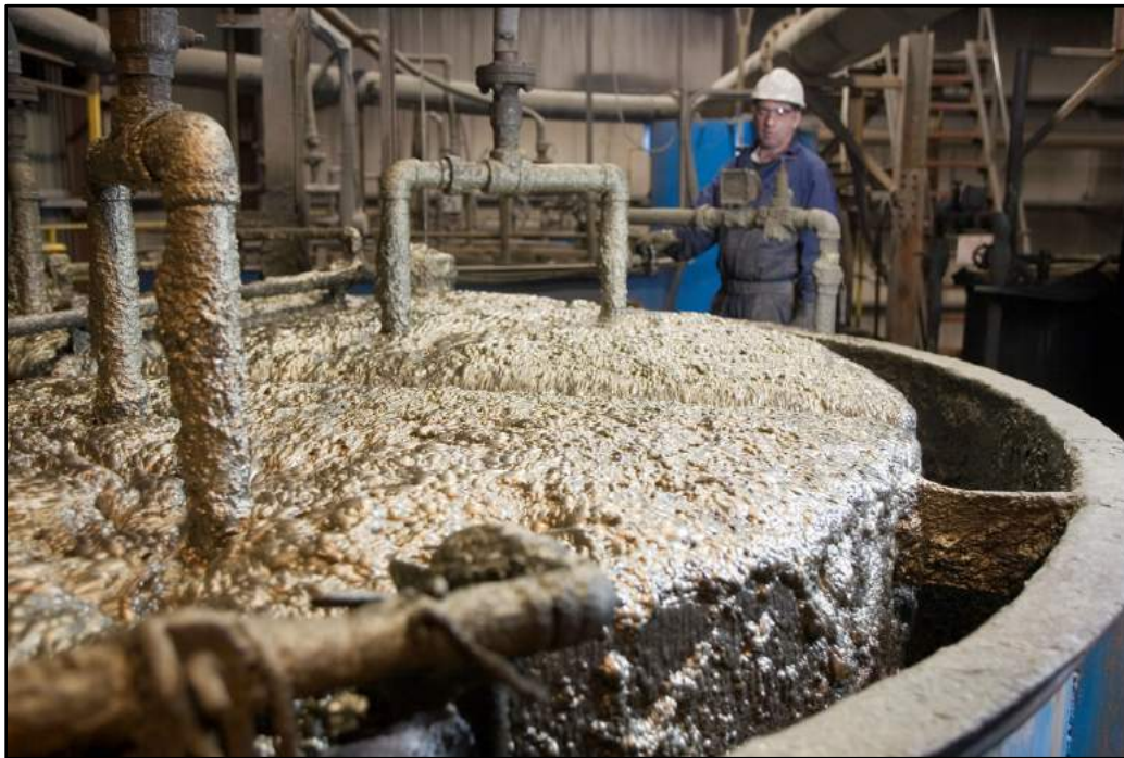
Figure 17-8 Mount Polley Mill Flotation Cell Producing Copper Concentrate
