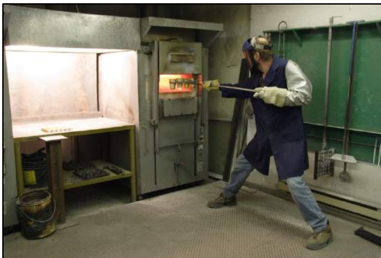
Figure 11-2 Fire Assaying at the Mount Polley Lab
