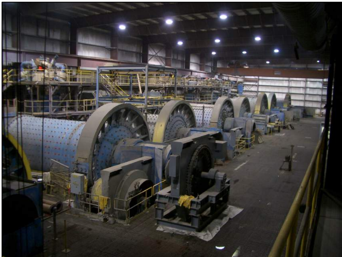
Figure 17-7 Mount Polley Rod, Ball and Pebble Mills
