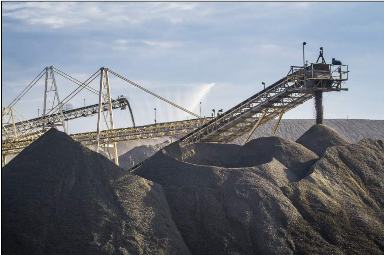
Figure 17-1 Mount Polley Mill Crushed Stockpile System
