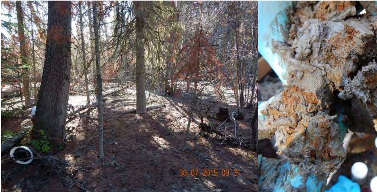
Figure 5: View of Plot 8 within the Halo Area and silty grey tailings (July 30, 2015). A soil test pit could not be dug because the tailings were saturated.
