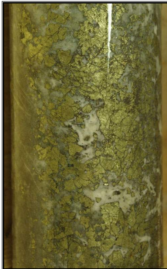
Figure 9.1 Red Chris Core Sample: Chalcopyrite in Quartz Stockwork
