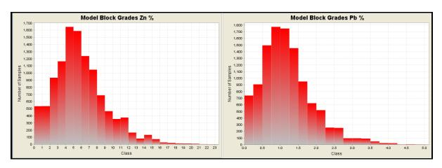
Figure 17-10 Block model frequency distribution of grades
