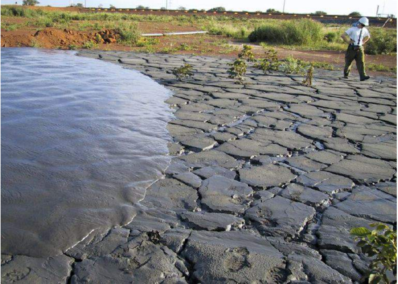
Figure 7: Paste Disposal at Bulyanhulu Gold Mine in Tanzania
