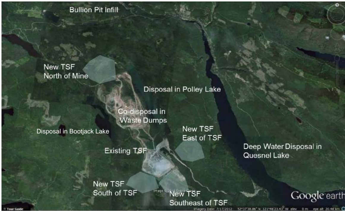
Figure 1: Potential Locations for a Future Tailings Storage Facility
