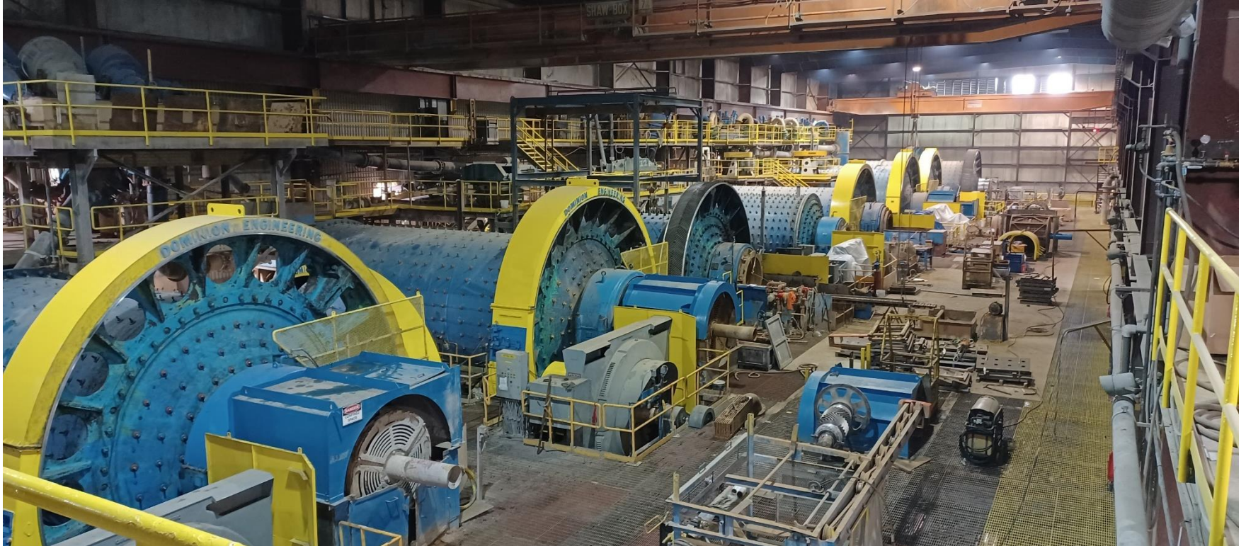
Grinding Circuit: three stage grinding circuit, two rod mills, three ball mills, and three pebble mills.
