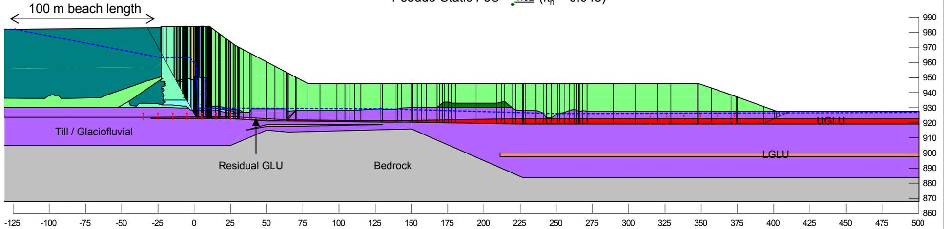
**Embankment configuration at tailings elevation 983 m**
