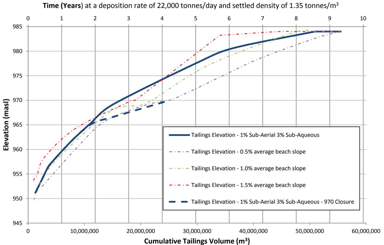
Figure 21: Tailings Storage Curves for Different Beach Slopes
