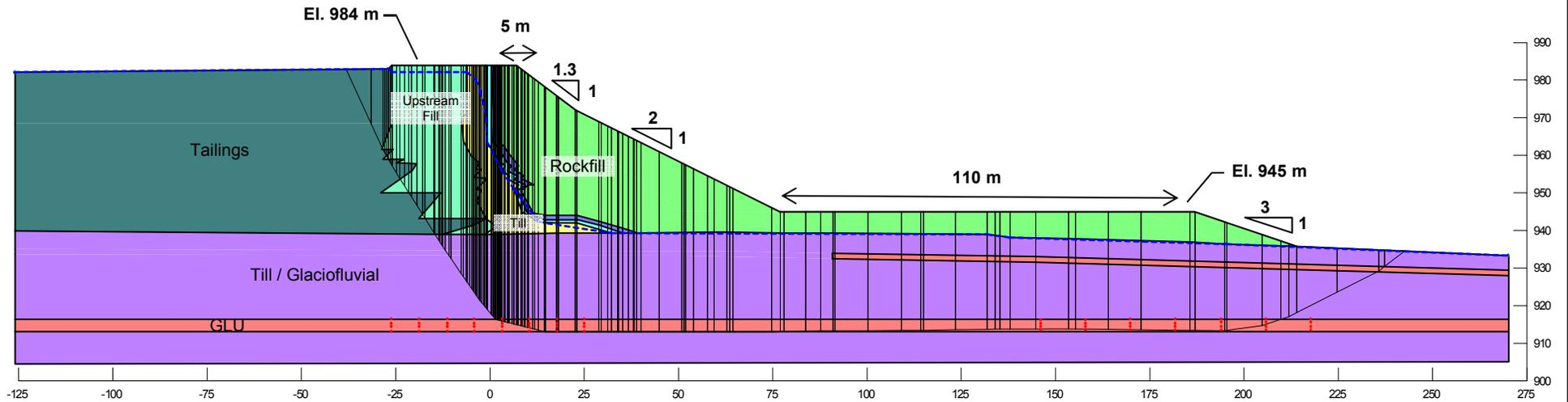
**Embankment configuration at tailings elevation 983 m**
