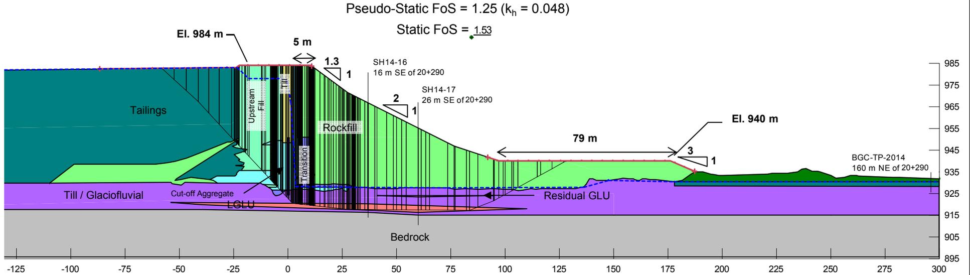
**Embankment configuration at tailings elevation 983 m**
