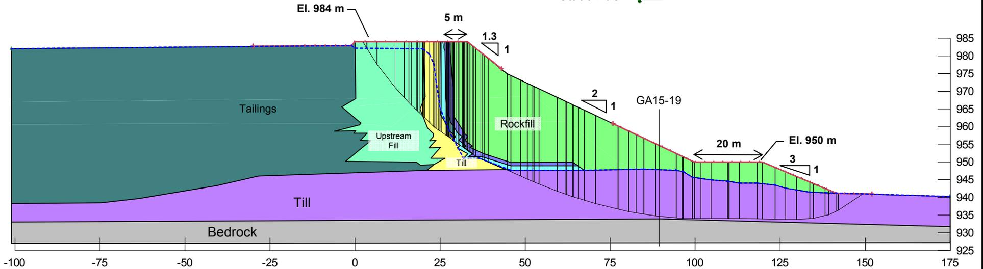
**Embankment configuration at tailings elevation 983 m**
