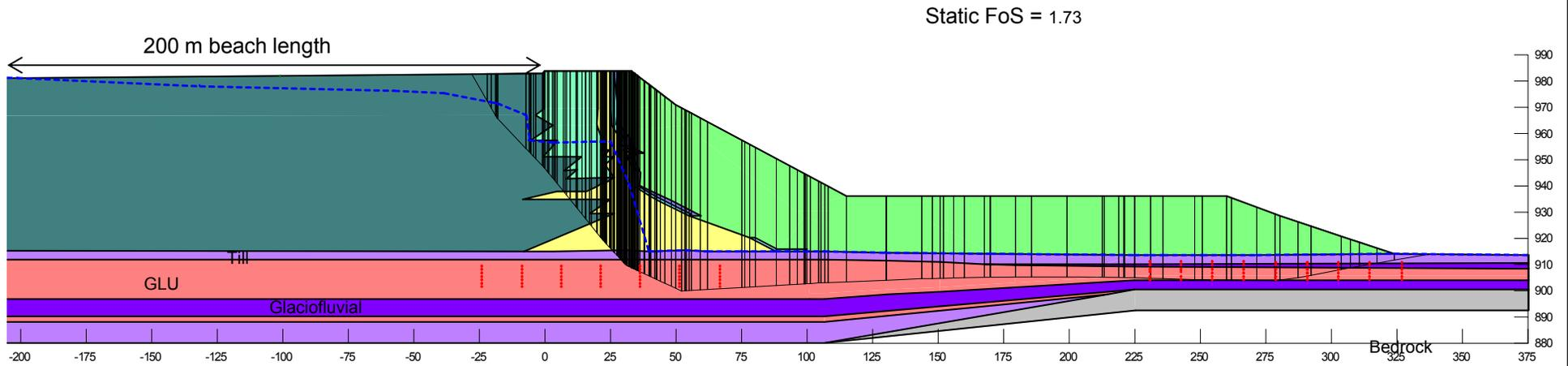
**Embankment configuration at tailings elevation 983 m**
