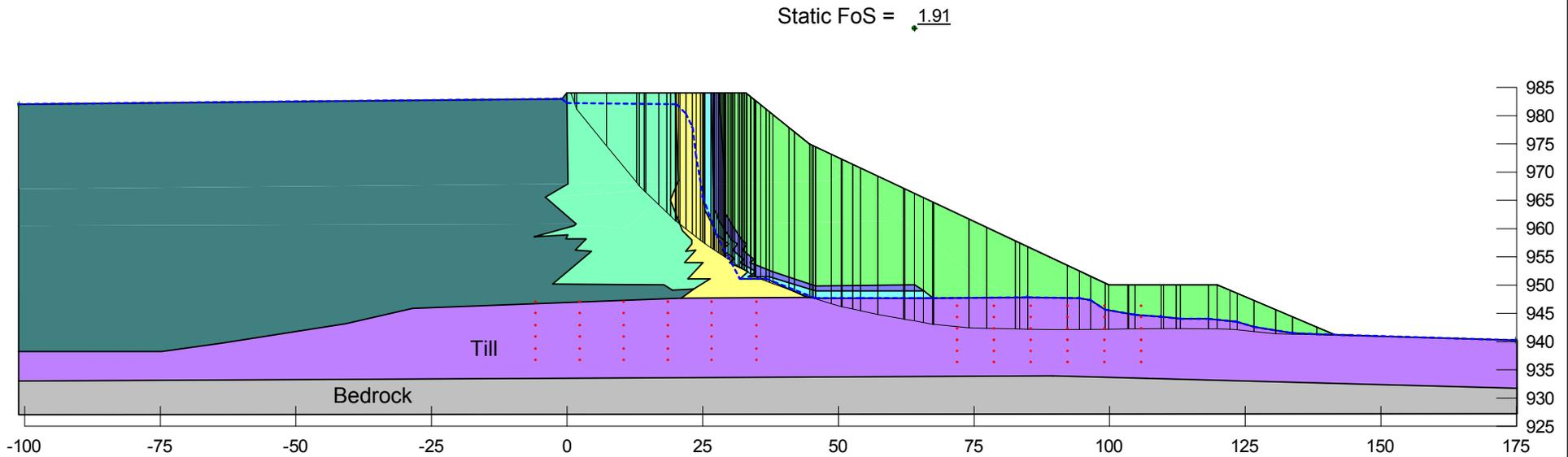
**Embankment configuration at tailings elevation 983 m**
