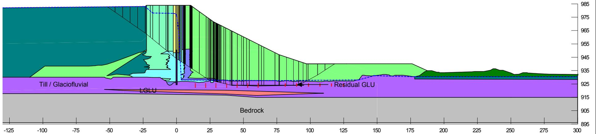
**Embankment configuration at tailings elevation 983 m**
