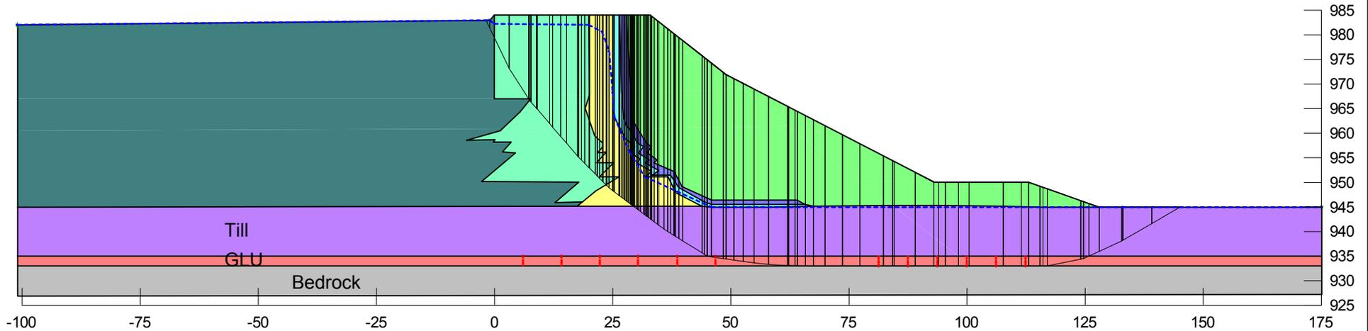
**Embankment configuration at tailings elevation 983 m**
