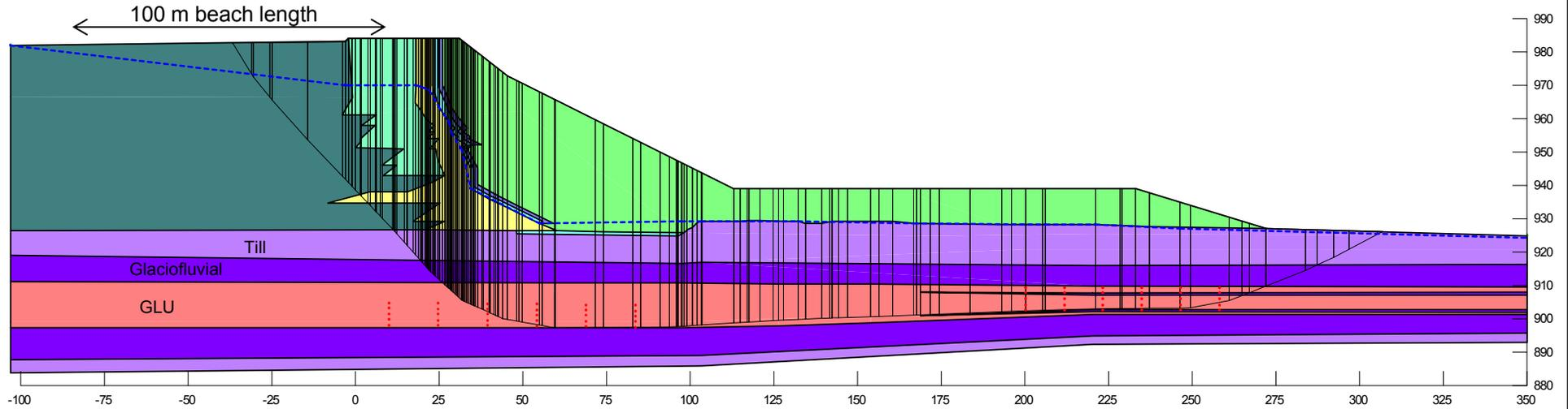
**Embankment configuration at tailings elevation 983 m**
