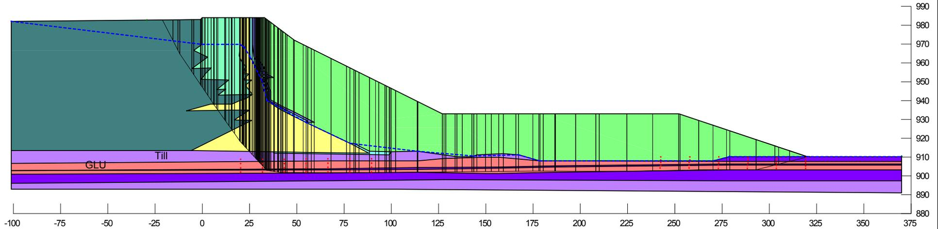
**Embankment configuration at tailings elevation 983 m**
