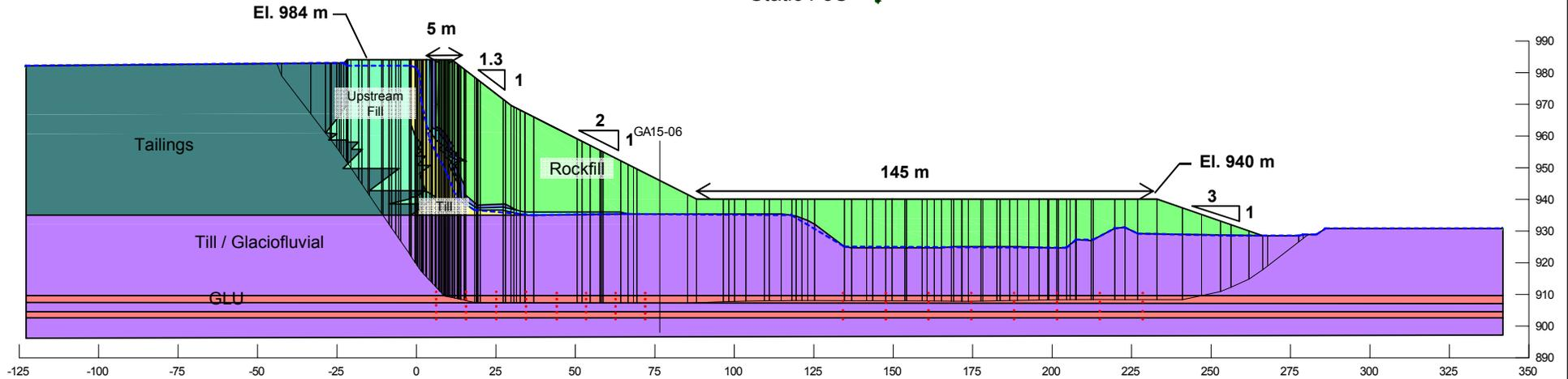
**Embankment configuration at tailings elevation 983 m**
