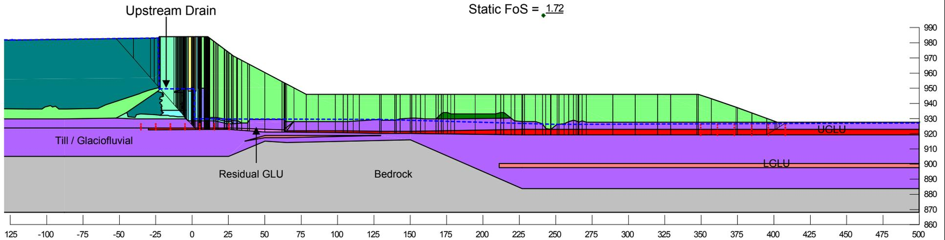
**Embankment configuration at tailings elevation 983 m**
