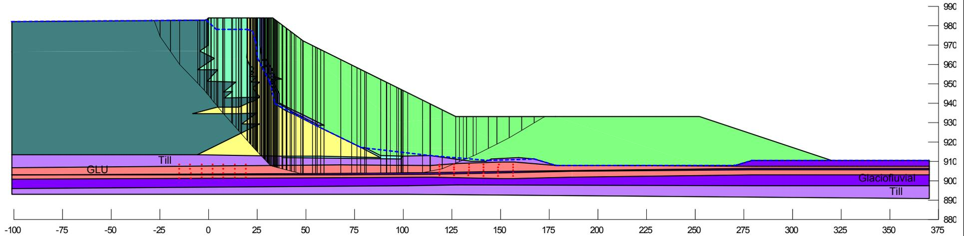
**Embankment configuration at tailings elevation 983 m**
