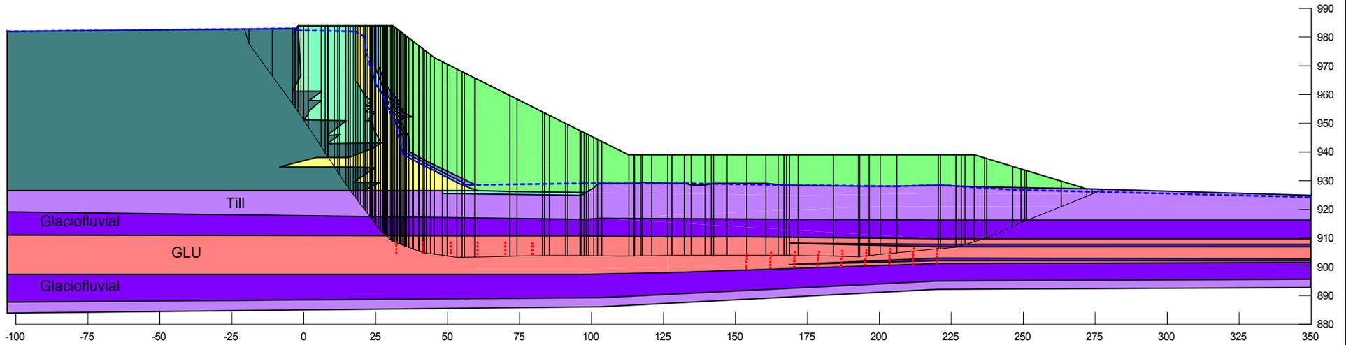
**Embankment configuration at tailings elevation 983 m**
