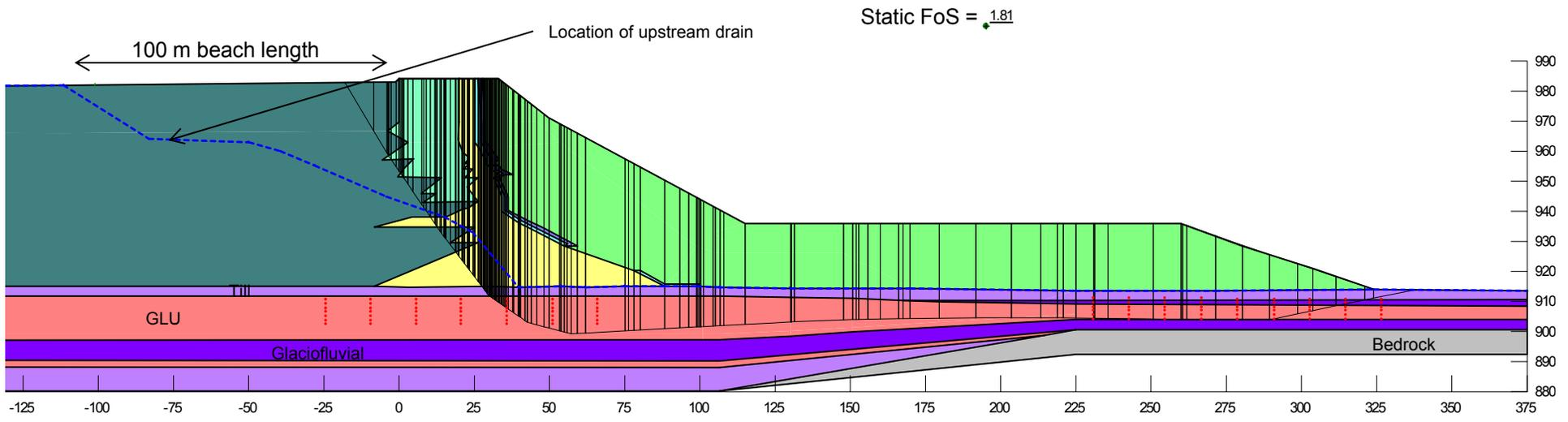
**Embankment configuration at tailings elevation 983 m**
