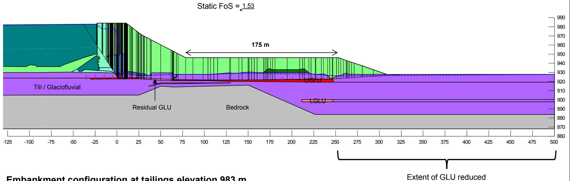
**Embankment configuration at tailings elevation 983 m**
