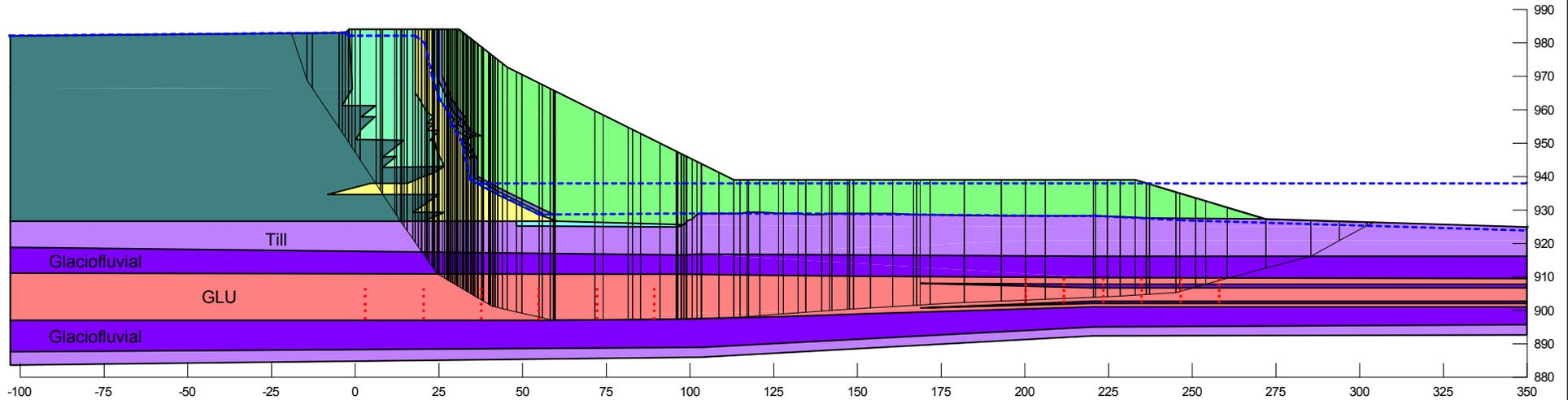
**Embankment configuration at tailings elevation 983 m**
