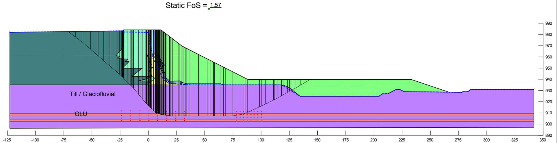
**Embankment configuration at tailings elevation 983 m**
