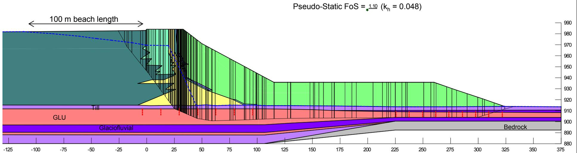
**Embankment configuration at tailings elevation 983 m**
