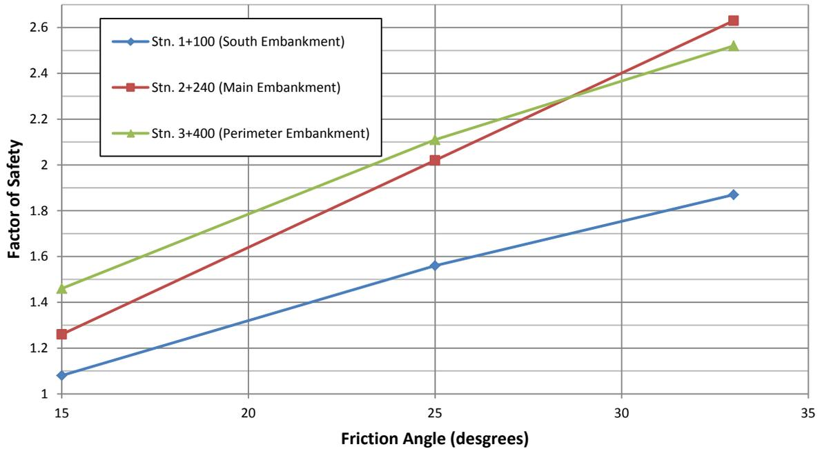
Figure 31: Factor of Safety vs Peak Friction Angle
