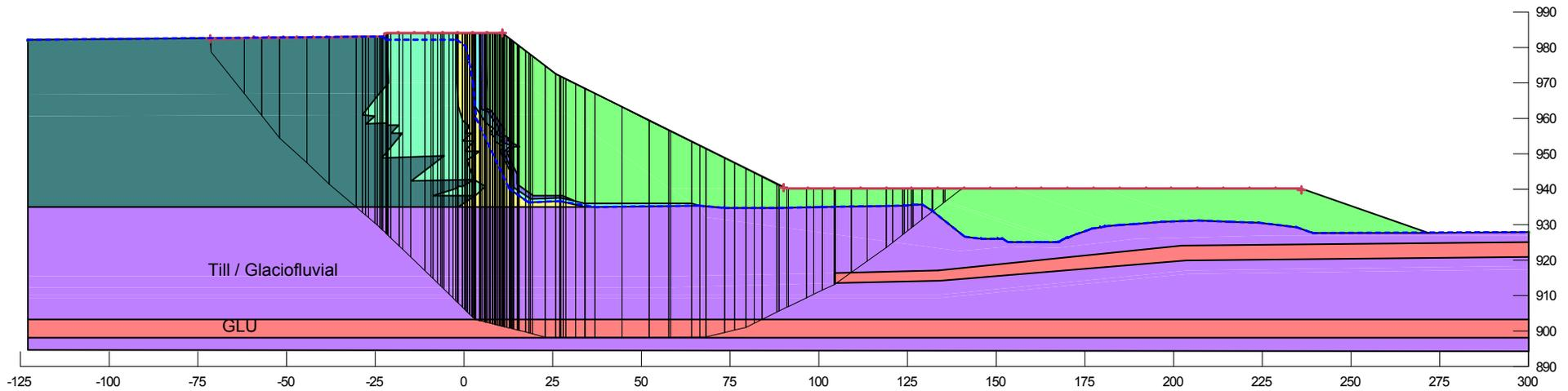
**Embankment configuration at tailings elevation 983 m**
