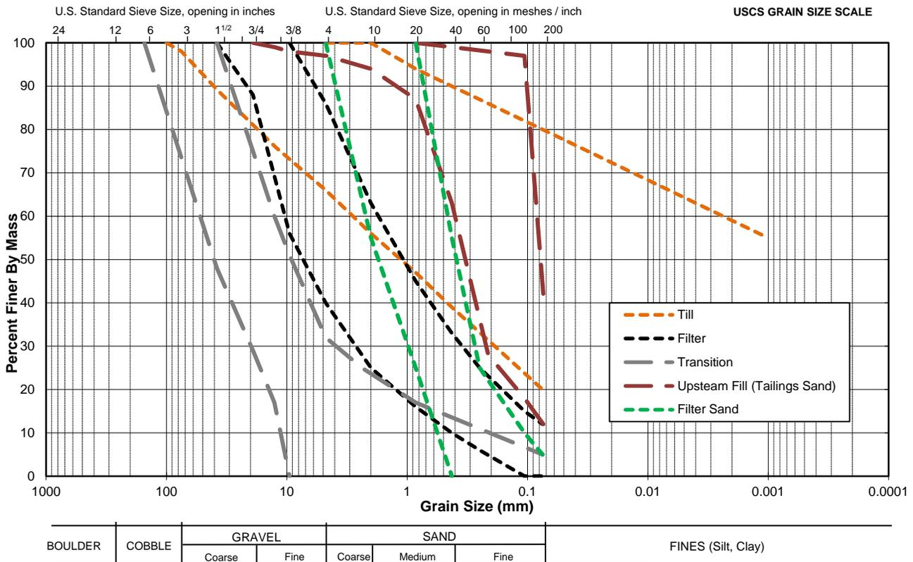
Figure 22: Proposed Construction Material Particle Size Distribution Envelopes
