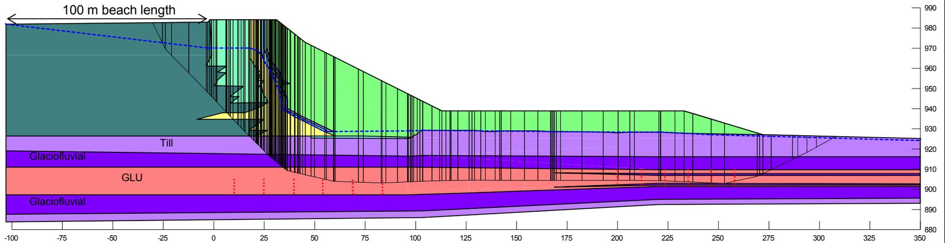
**Embankment configuration at tailings elevation 983 m**
