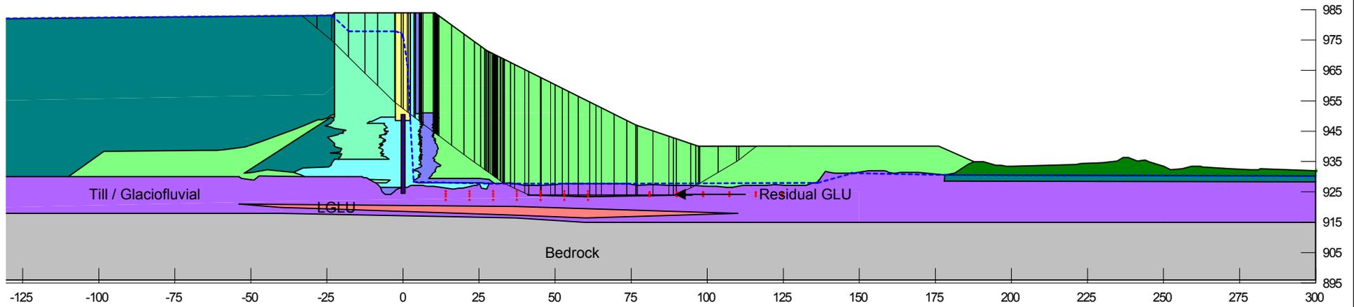
**Embankment configuration at tailings elevation 983 m**
