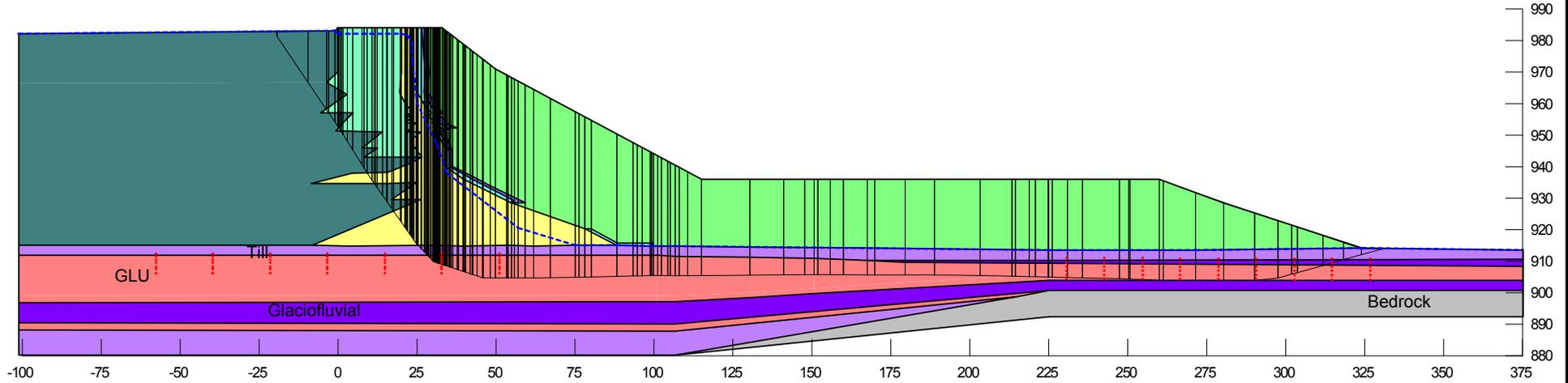
**Embankment configuration at tailings elevation 983 m**
