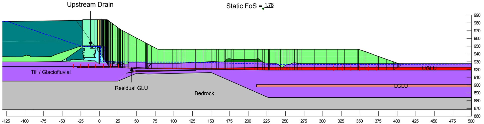
**Embankment configuration at tailings elevation 983 m**
