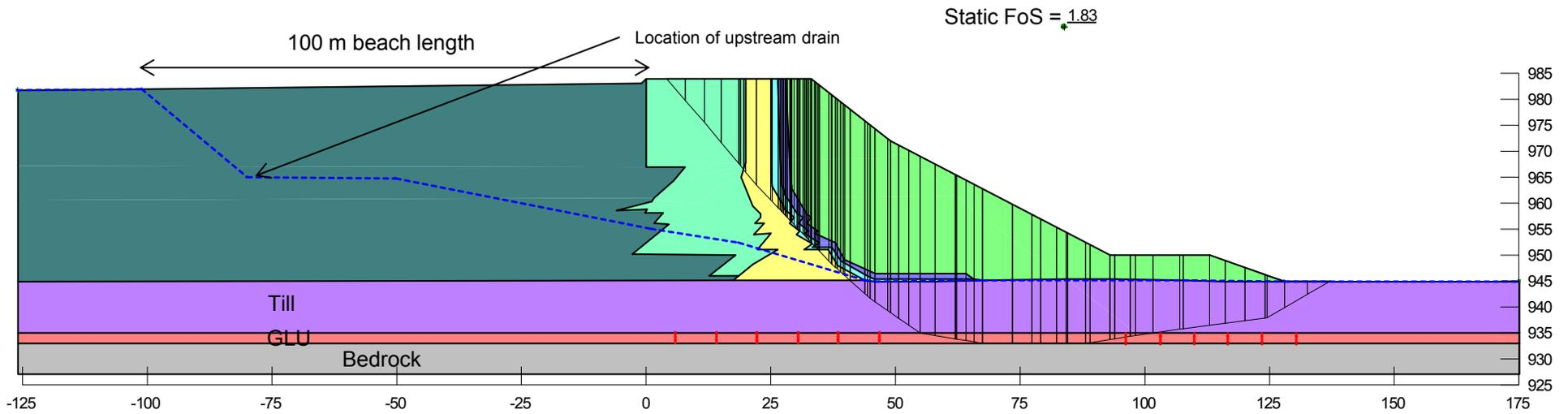
**Embankment configuration at tailings elevation 983 m**
