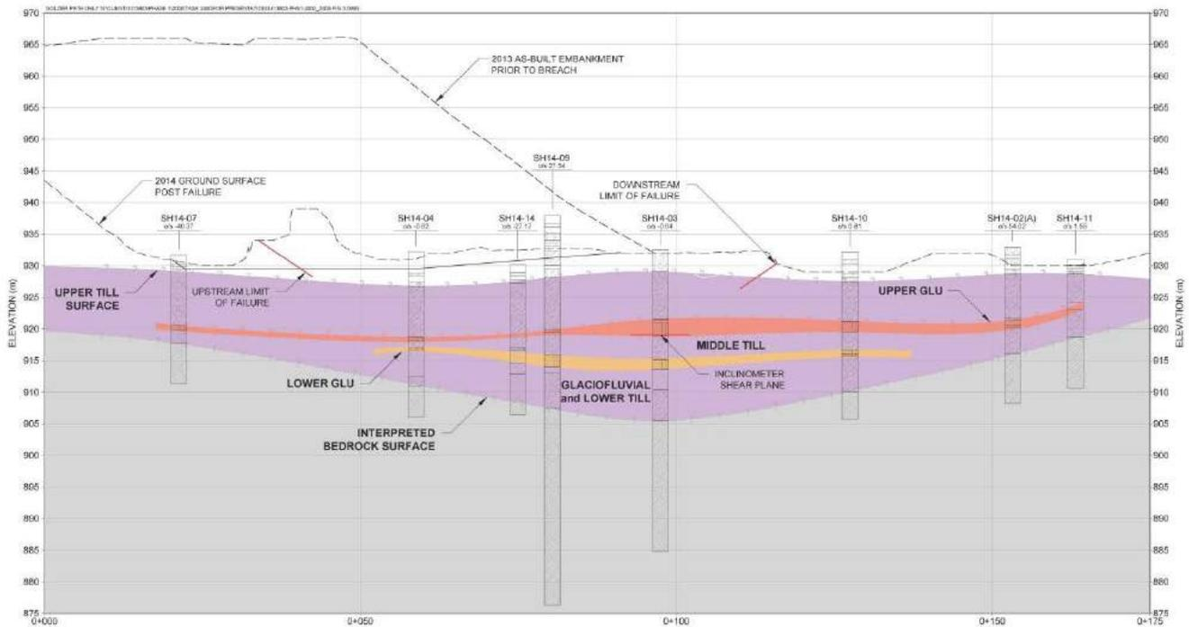
Figure 3: Typical Soil Stratigraphy at Corner 1
