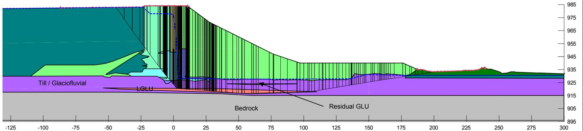
**Embankment configuration at tailings elevation 983 m**
