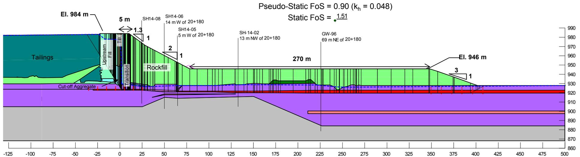
**Embankment configuration at tailings elevation 983 m**
