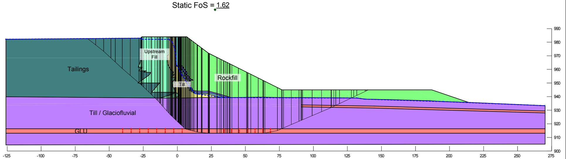
**Embankment configuration at tailings elevation 983 m**
