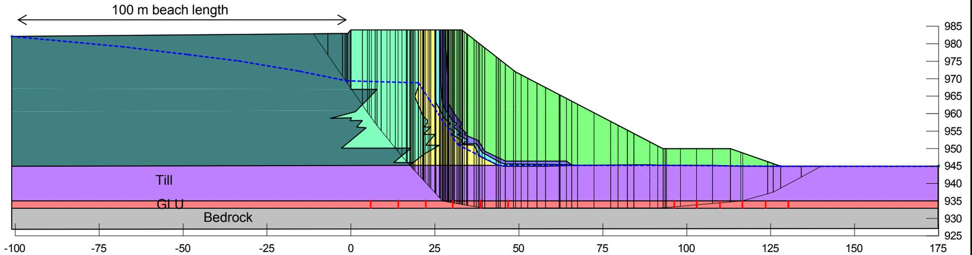
**Embankment configuration at tailings elevation 983 m**
