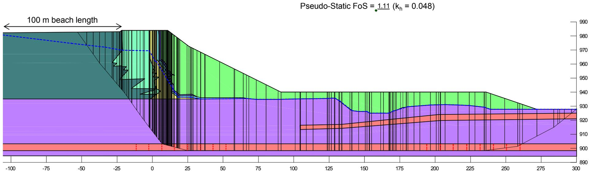
**Embankment configuration at tailings elevation 983 m**
