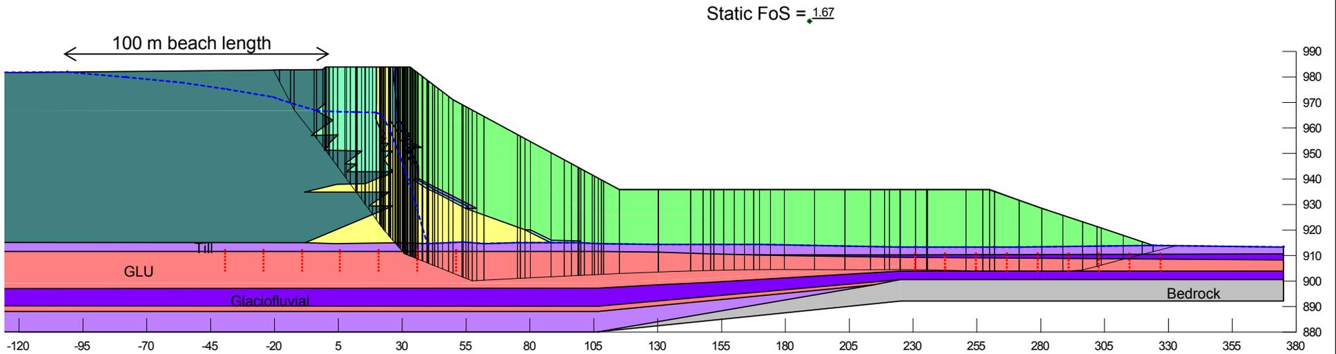
**Embankment configuration at tailings elevation 983 m**
