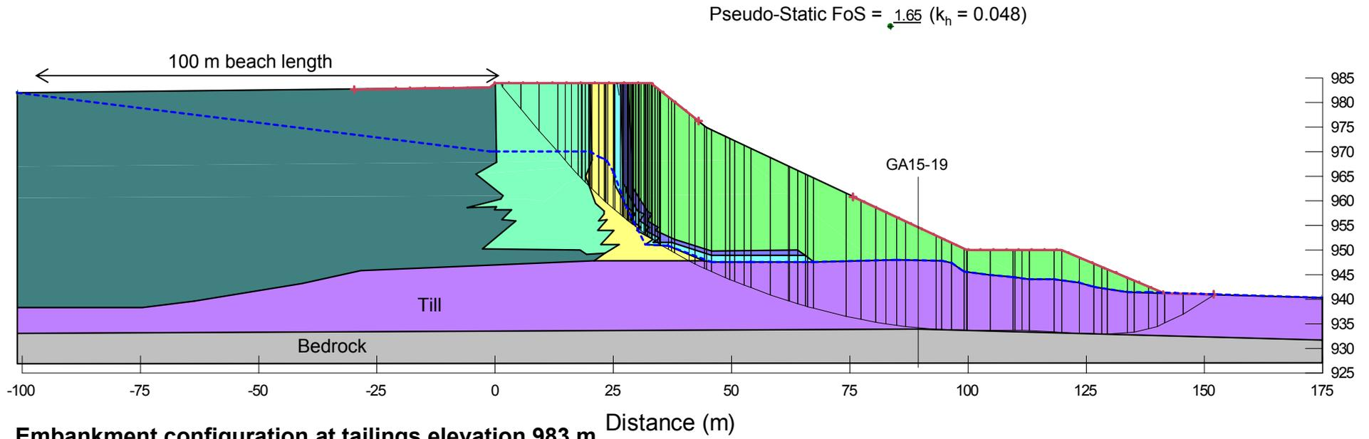
**Embankment configuration at tailings elevation 983 m**
