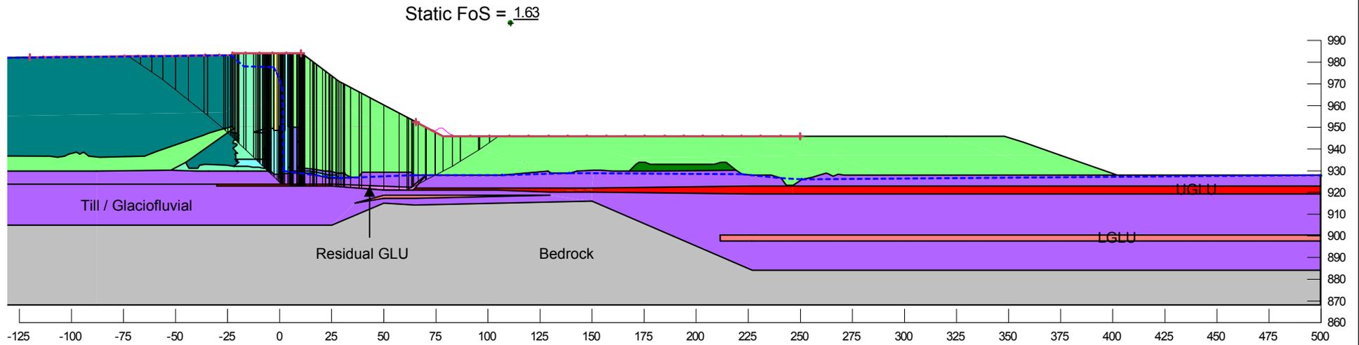
**Embankment configuration at tailings elevation 983 m**
