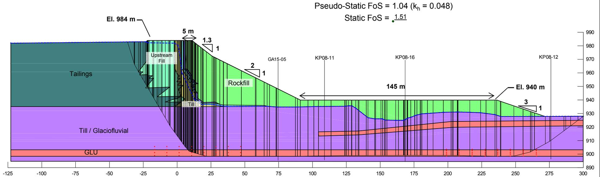
**Embankment configuration at tailings elevation 983 m**
