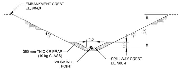
SCALE 1:100 m **A** SPILLWAY CREST SECTION
