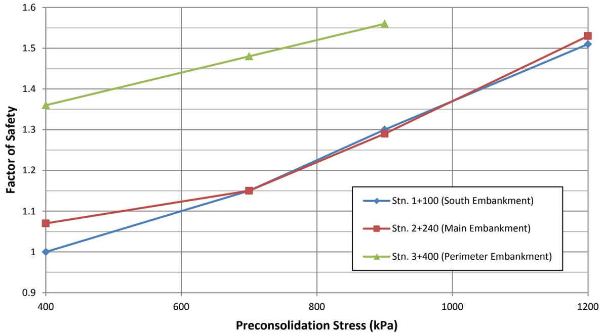
Figure 30: Factor of Safety vs Preconsolidation Stress
