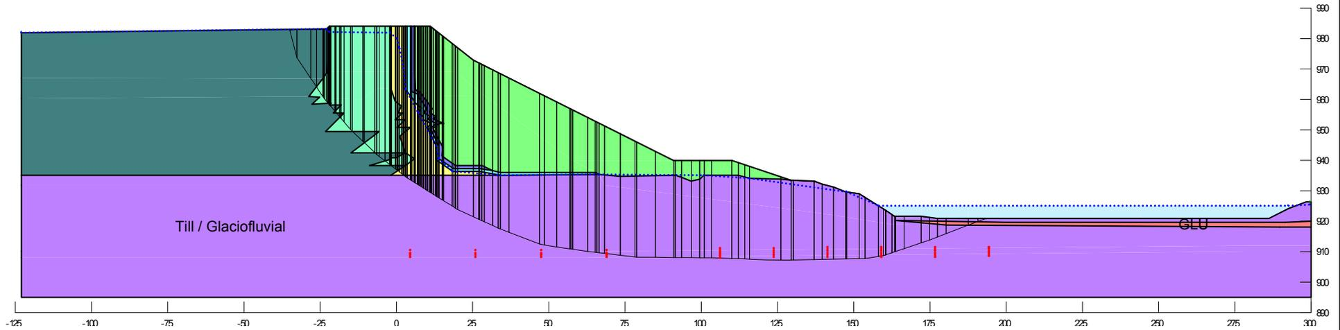
**Embankment configuration at tailings elevation 983 m**
