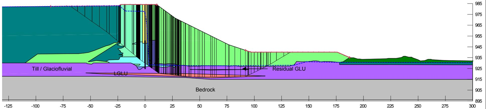
**Embankment configuration at tailings elevation 983 m**
