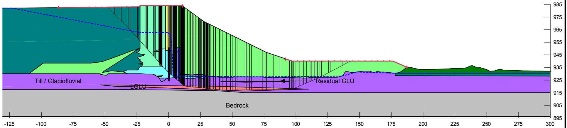
**Embankment configuration at tailings elevation 983 m**
