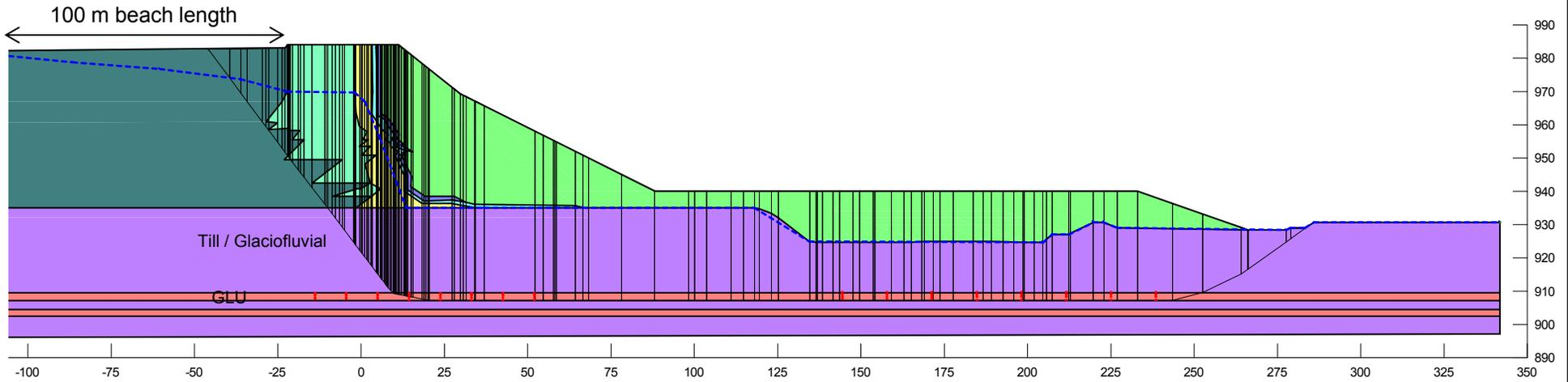
**Embankment configuration at tailings elevation 983 m**
