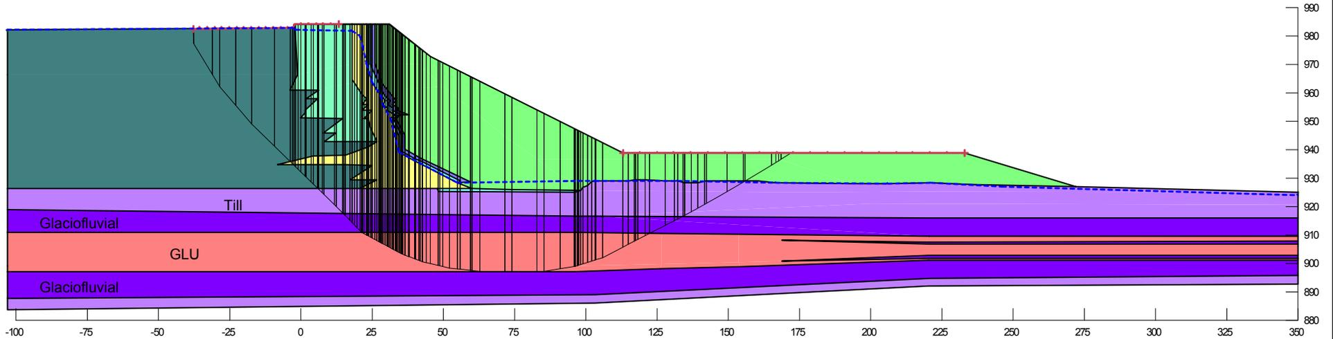
**Embankment configuration at tailings elevation 983 m**
