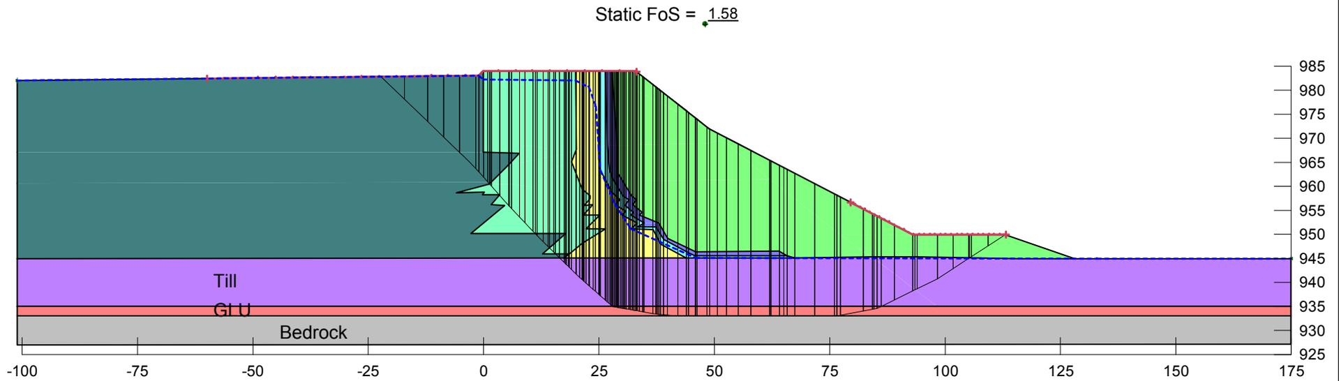
**Embankment configuration at tailings elevation 983 m**
