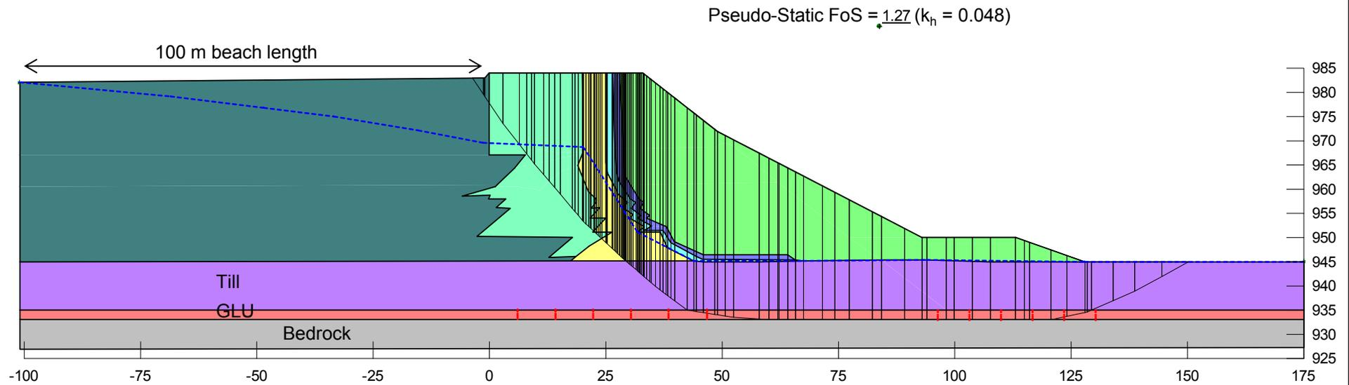
**Embankment configuration at tailings elevation 983 m**
