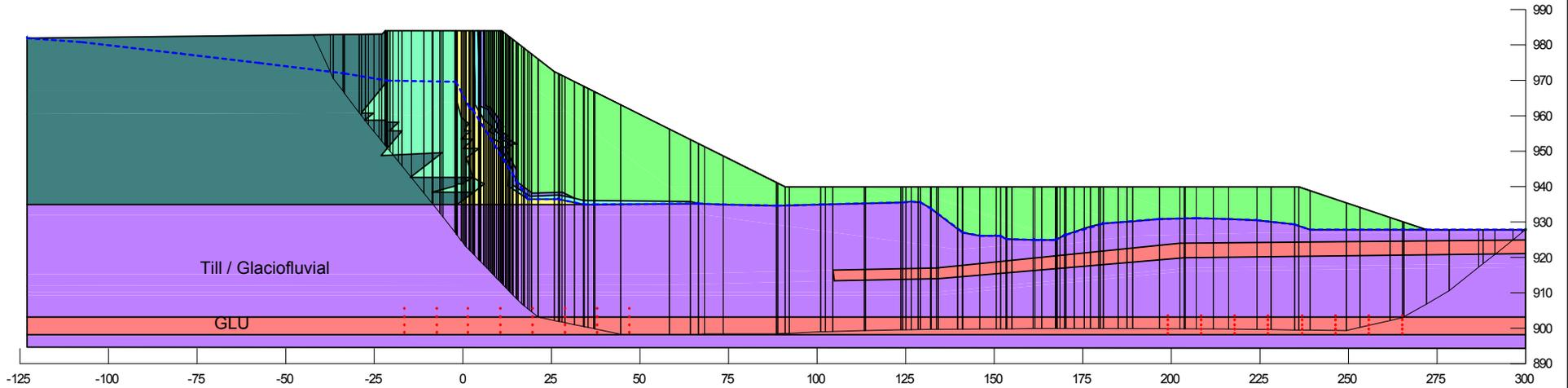
**Embankment configuration at tailings elevation 983 m**
