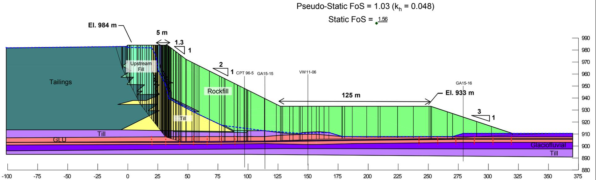
**Embankment configuration at tailings elevation 983 m**
