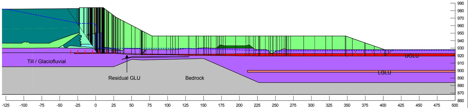
**Embankment configuration at tailings elevation 983 m**
