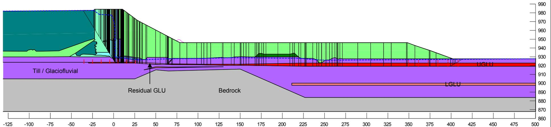
**Embankment configuration at tailings elevation 983 m**
