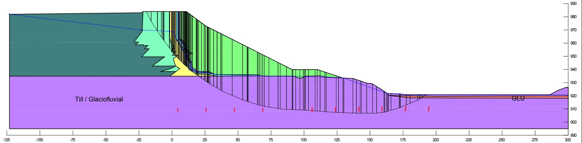
**Embankment configuration at tailings elevation 983 m**
