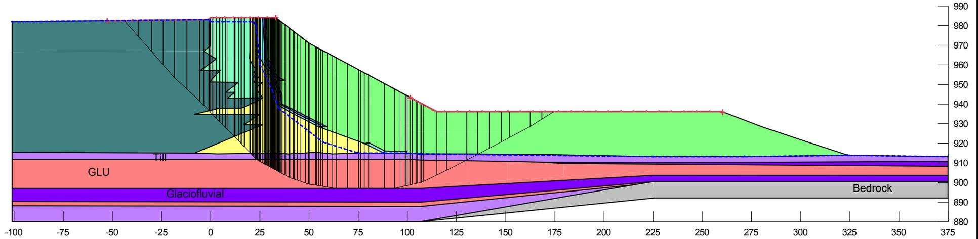
**Embankment configuration at tailings elevation 983 m**
