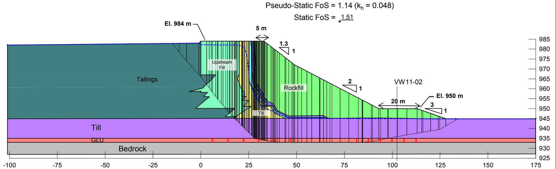
**Embankment configuration at tailings elevation 983 m**
