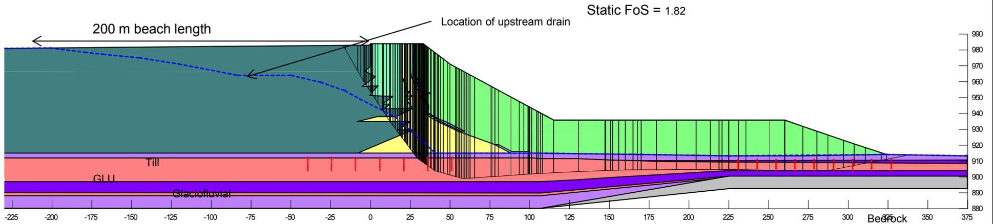
**Embankment configuration at tailings elevation 983 m**
