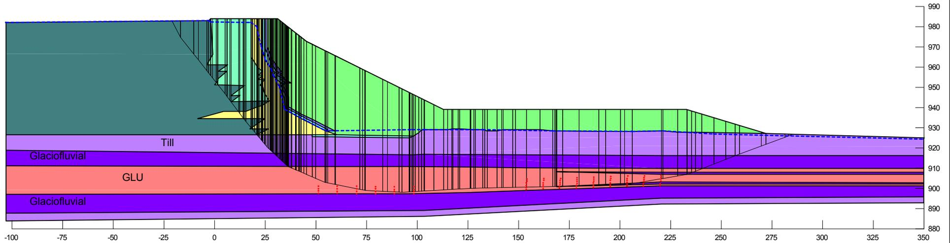
**Embankment configuration at tailings elevation 983 m**
