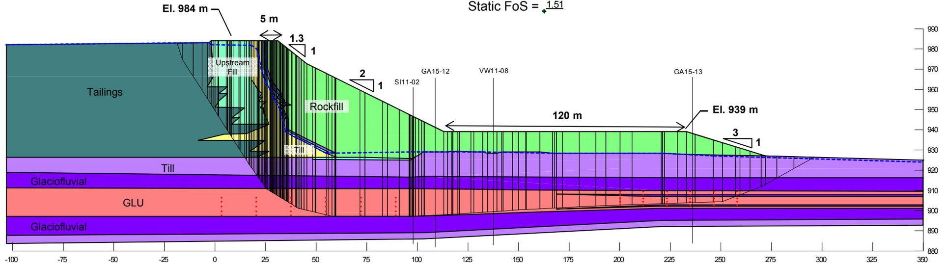
**Embankment configuration at tailings elevation 983 m**
