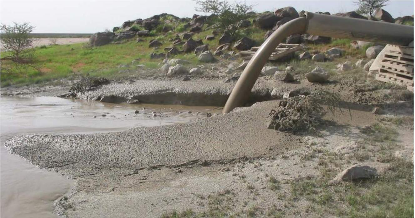
*Figure 5: Discharge of Thickened Tailings (Essakane Gold Mine)*
