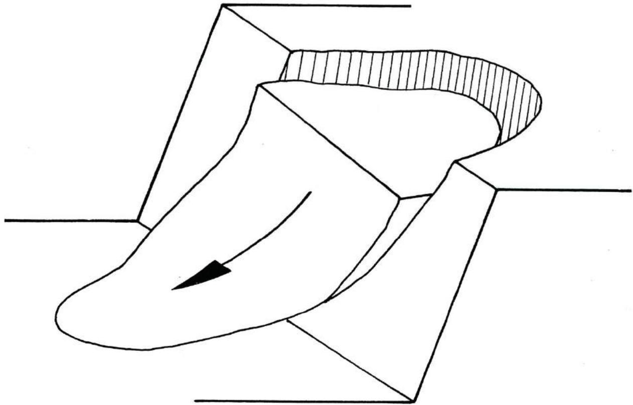
*Quasi-Circular Failure in Weak or Heavily Fractured Rock*
