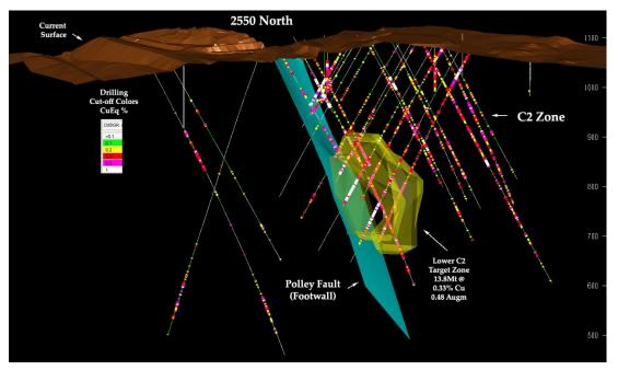
• WX and C2 Drill Targets-This figure shows the drill target zone. The Polley fault is blue.
