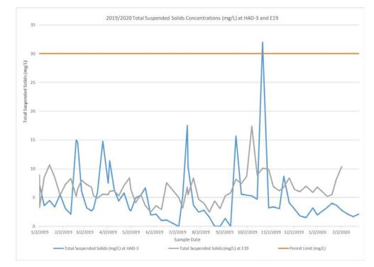
• Water treatment plant – influent (E19) vs effluent (HAD3); TSS, total copper and total selenium.
