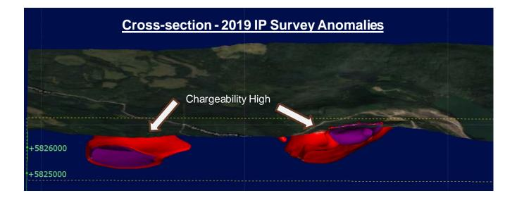
• Combination of magnetic and chargeable high. The green labelled lines are sites of potential diamond drill holes included in the Notice of Work (NOW) that has been submitted.
