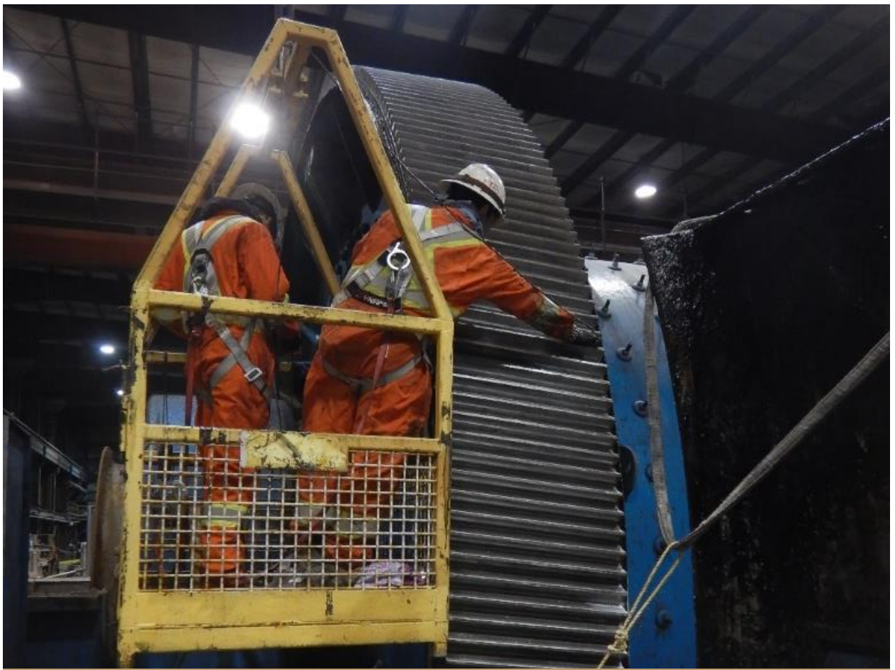
Figure 7 Staff assessing mill gear teeth
