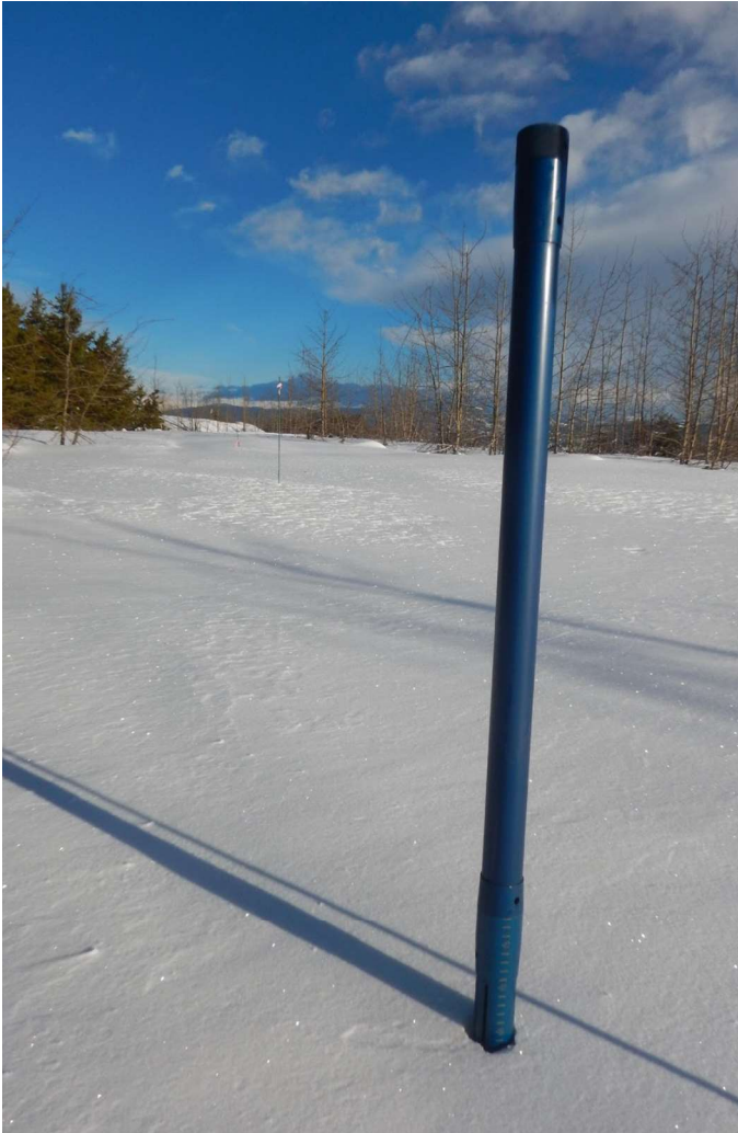
Figure 1 Snow corer for evaluating snowpack.
