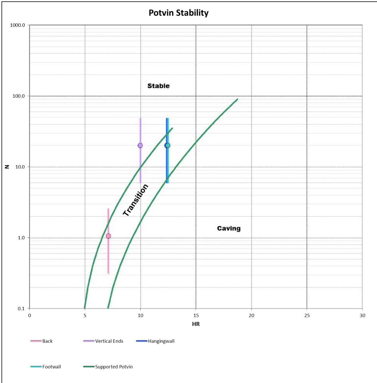
Figure 7: Plot of Block B and C Mined Together on the Potvin Stability Graph (Assumes Supported Slope Walls)
