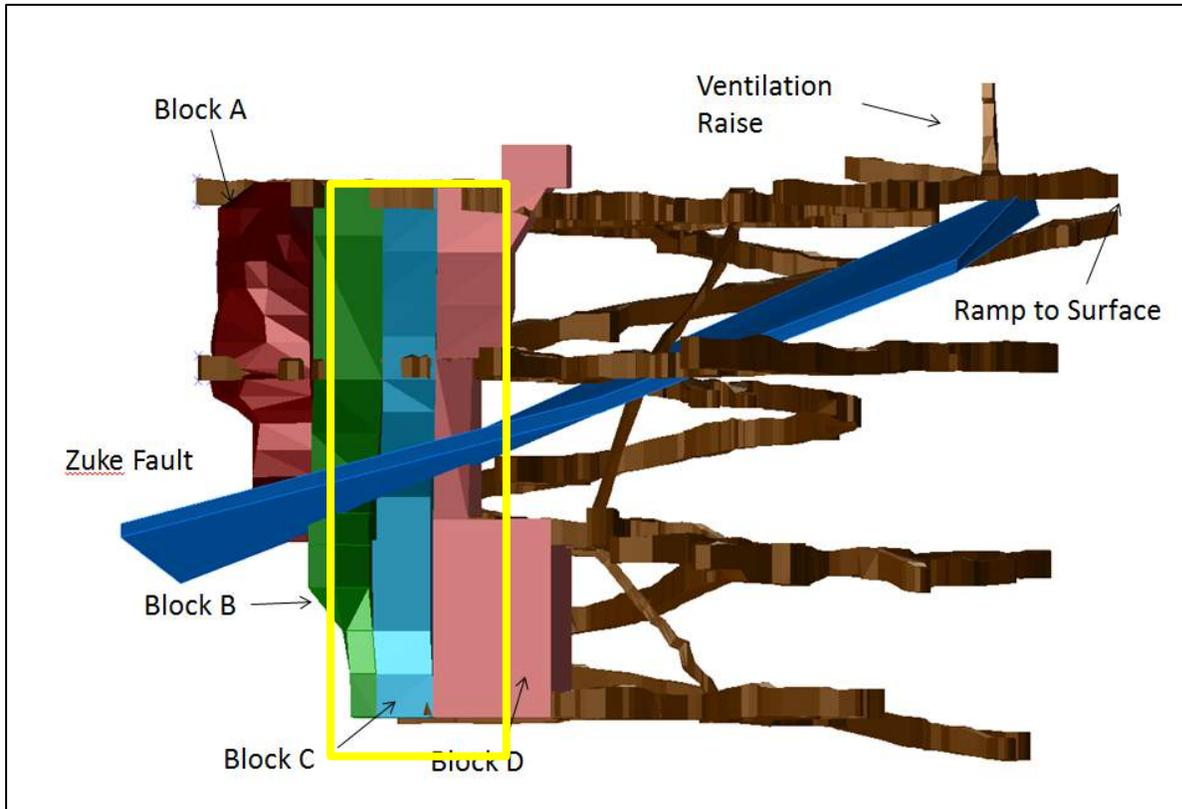
Figure 1: Longitudinal Section of the Boundary Zone Showing the Stopping Blocks and Development
