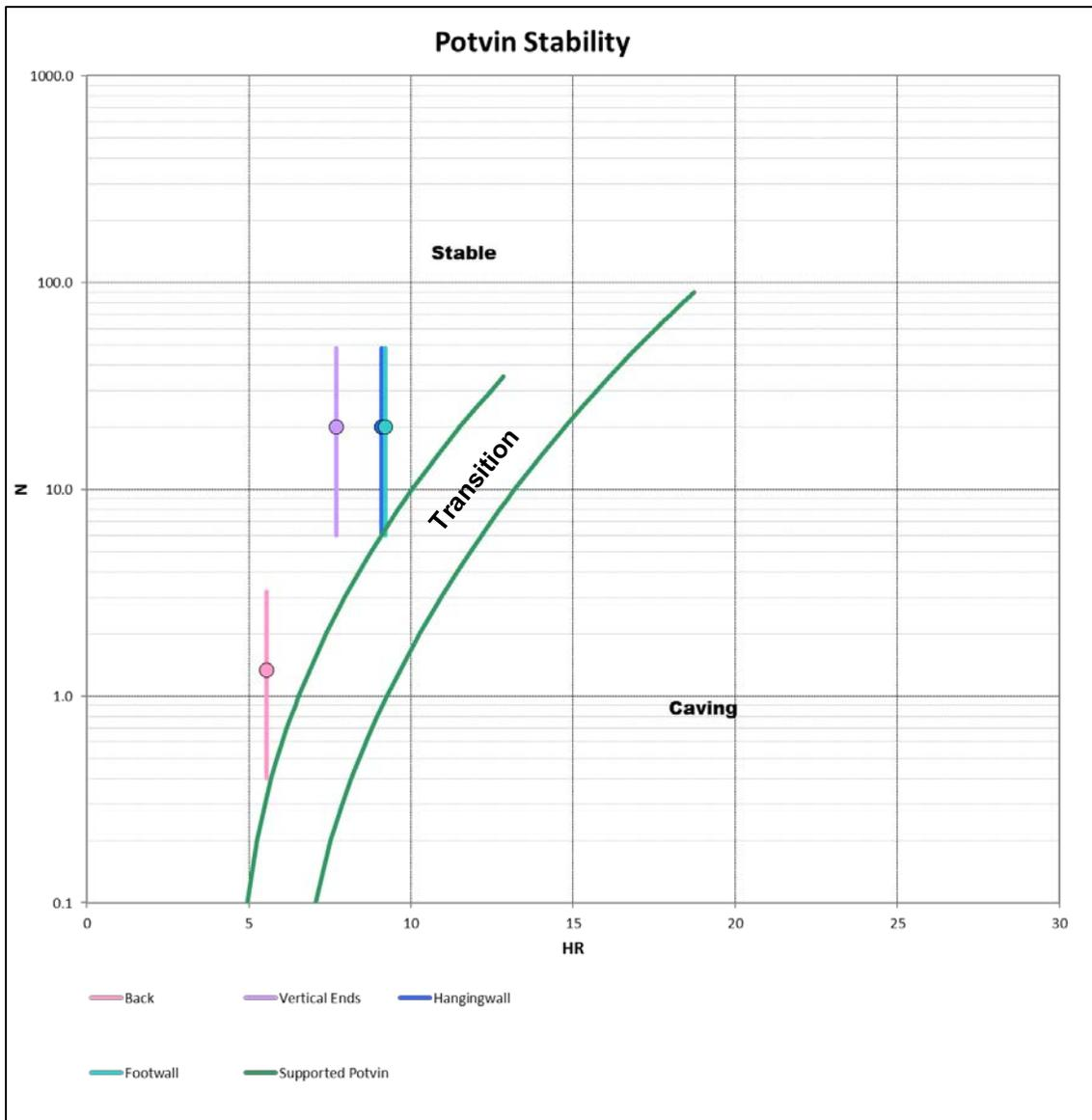
Figure 6: Plot of Block A on the Potvin Stability Graph (Assumes Supported Stope Walls)
