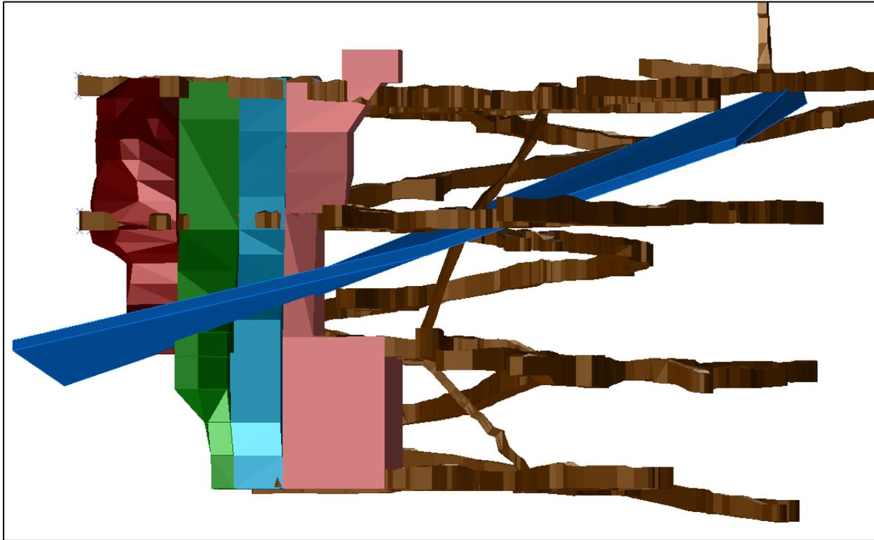
Figure 3: Longitudinal Section Showing the Location of the Zuke Fault Relative to the Stopping Blocks
