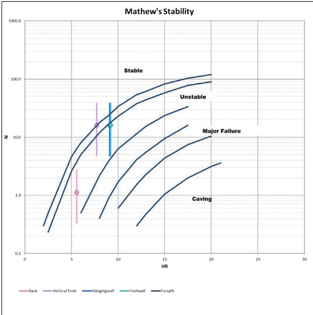
Figure 5: Plot of Block A on the Mathews Stability Graph (Assumes Unsupported Slope Walls)
