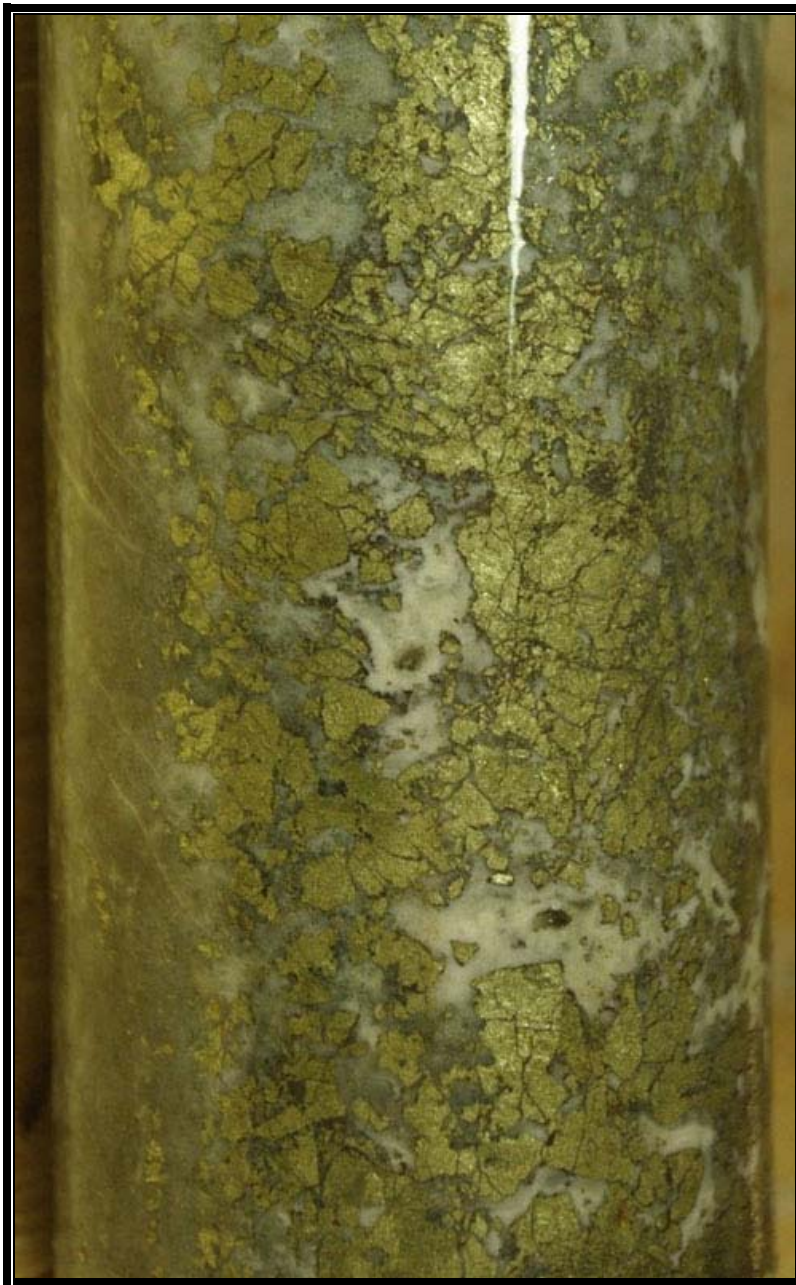
Figure 9.4 Red Chris Core Sample: Chalcopyrite in Quartz Stockwork
