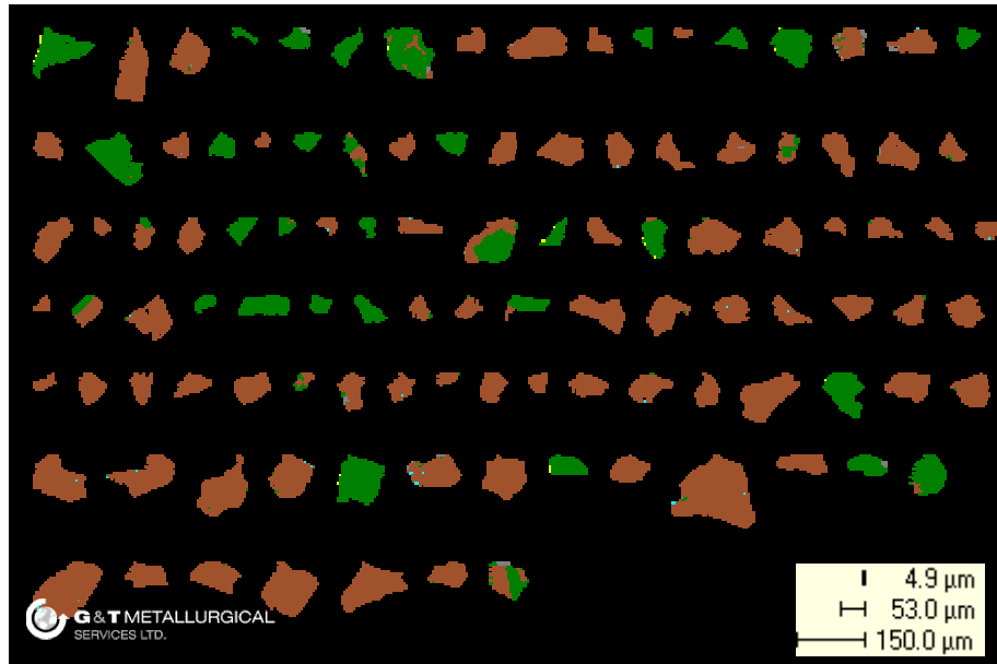
Examples of Liberated Chalcopyrite and Bornite
