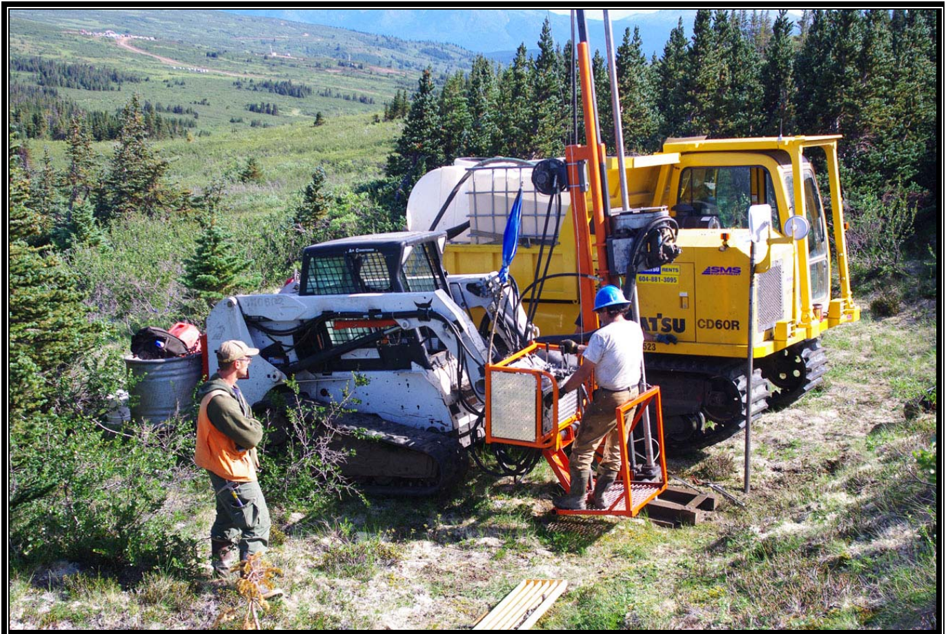
Figure 11.3 Bobcat Mounted Hydra Core Drill
