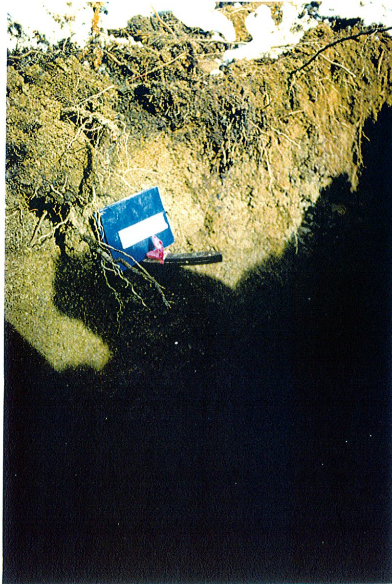
Figure 2: Soil pit #MP95-12a: Luvisolic soil developed on deep, calcareous till parent material.
