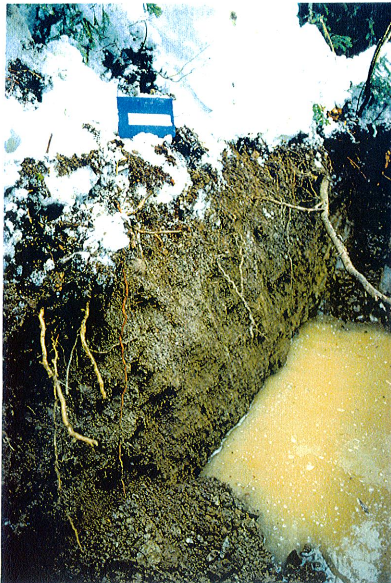
Figure 6: Soil pit #MP95-16a: Podzolic gray luvisol on a morainal veneer over rock. The till in this area was up to 20' thick.
