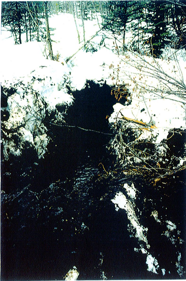
Figure 7: Soil pit #MP95-17: Typic mesisol organic soil formed over a poorly drained glacio-lacustrine parent material.
