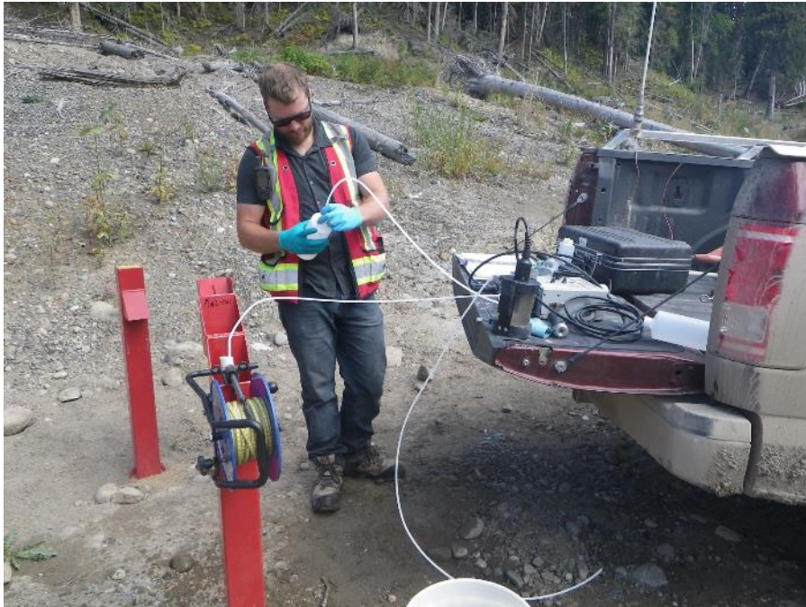
Photograph 7: Groundwater Sampling Of MW16-06S
