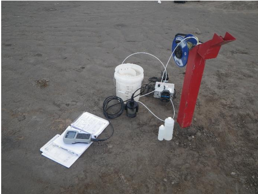
Photograph 5: Groundwater Sampling Set-Up at MW16-02
