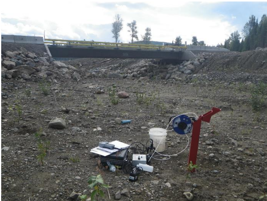
Photograph 6: Groundwater Sampling Set-Up at MW16-07
