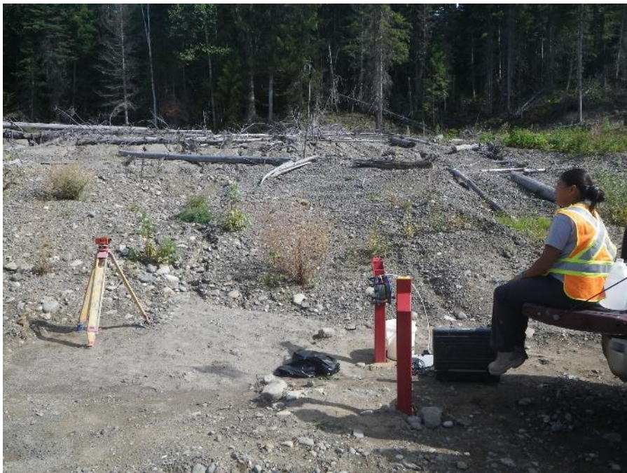
Photograph 8: Surveying Wells after Sampling Groundwater
