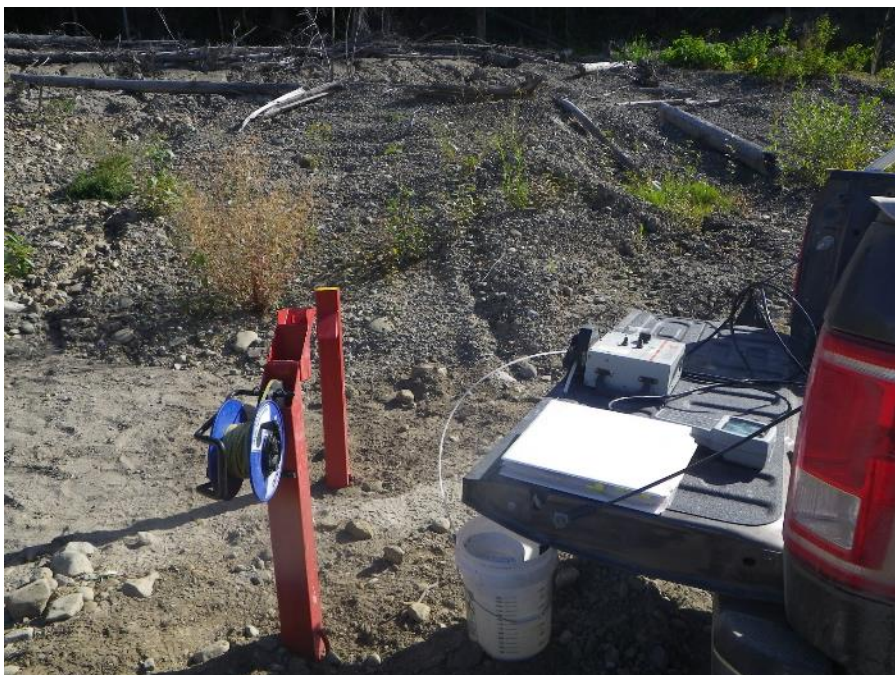
Photograph 4: Developing MW16-06S using a Peristaltic Pump
