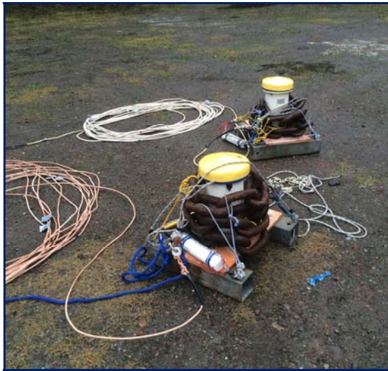
These acoustic doppler current profilers (ACDP) use the variable nature of sound waves created by particles in the water to measure water currents. They are also instrumented with temperature and turbidity probes and double as anchors for two of the moorings. Photo: S. Albers, QRRC Manager
