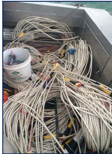
The heavily instrumented moorings prior to deployment on UNBC's Mathews research vessel. Moorings are anchored to the lake bottom by a heavy chain and submerged just below the surface. The moorings provide continuous information on the physical structure and biological patterns within Quesnel Lake. Photo: S. Albers, QRRC Manager
